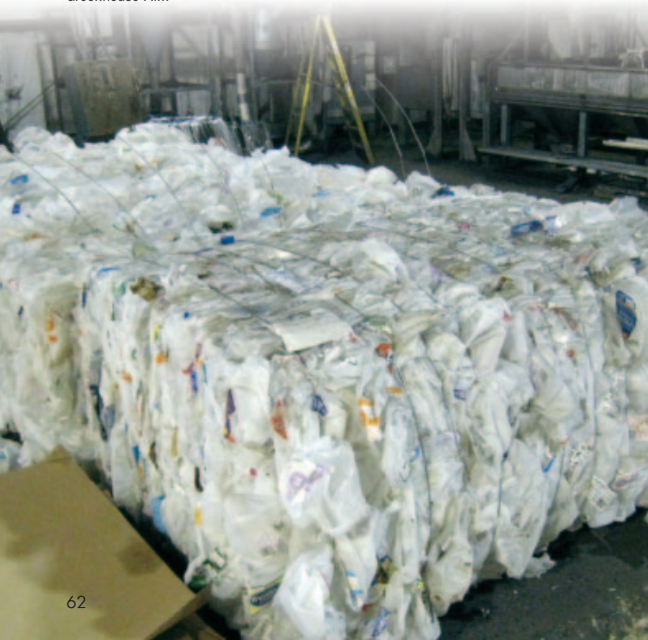
Figure 1: Baled LDPE Greenhouse Film
