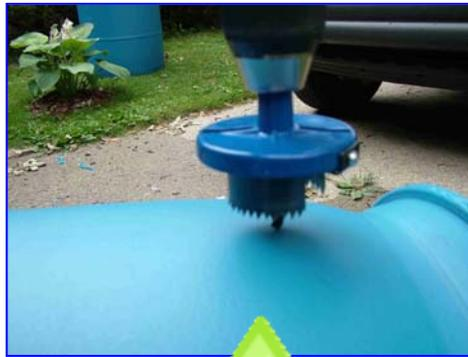
3. Drill hole for overflow near the top, on the side you prefer. For regular faucet, use a 1" drill bit. For the PVC insert, use the 1<sup>3</sup>/<sub>4</sub> hole saw. Screw in fixture. Attach sprinkler hose to PVC, or regular garden hose to faucet. Overflow water should be drained away from the foundation of your home. If you are attaching two barrels together, attach PVC inserts to both barrels and join with hose.
