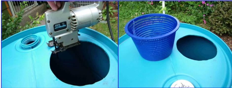
1. Trace the outside of the strainer basket. If basket has a "lip", then measure width of lip and cut the hole that much smaller. Drill 1" hole then use saber saw to cut basket opening.
